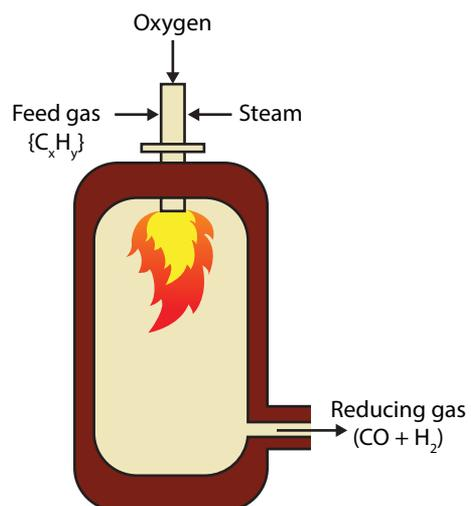
Production of reducing gas by partial oxidation
