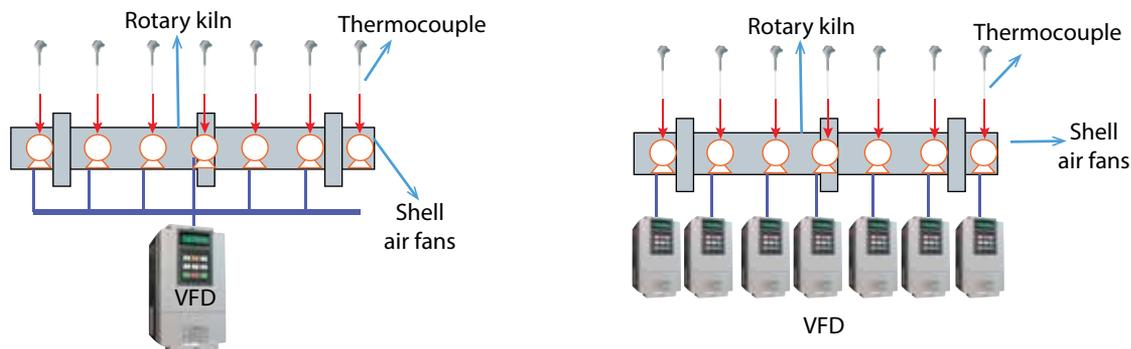
Decentralized VFD system in rotary kiln
