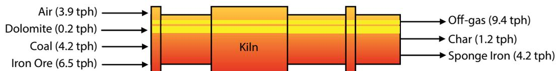
Mass balance of a coal-based rotary kiln
