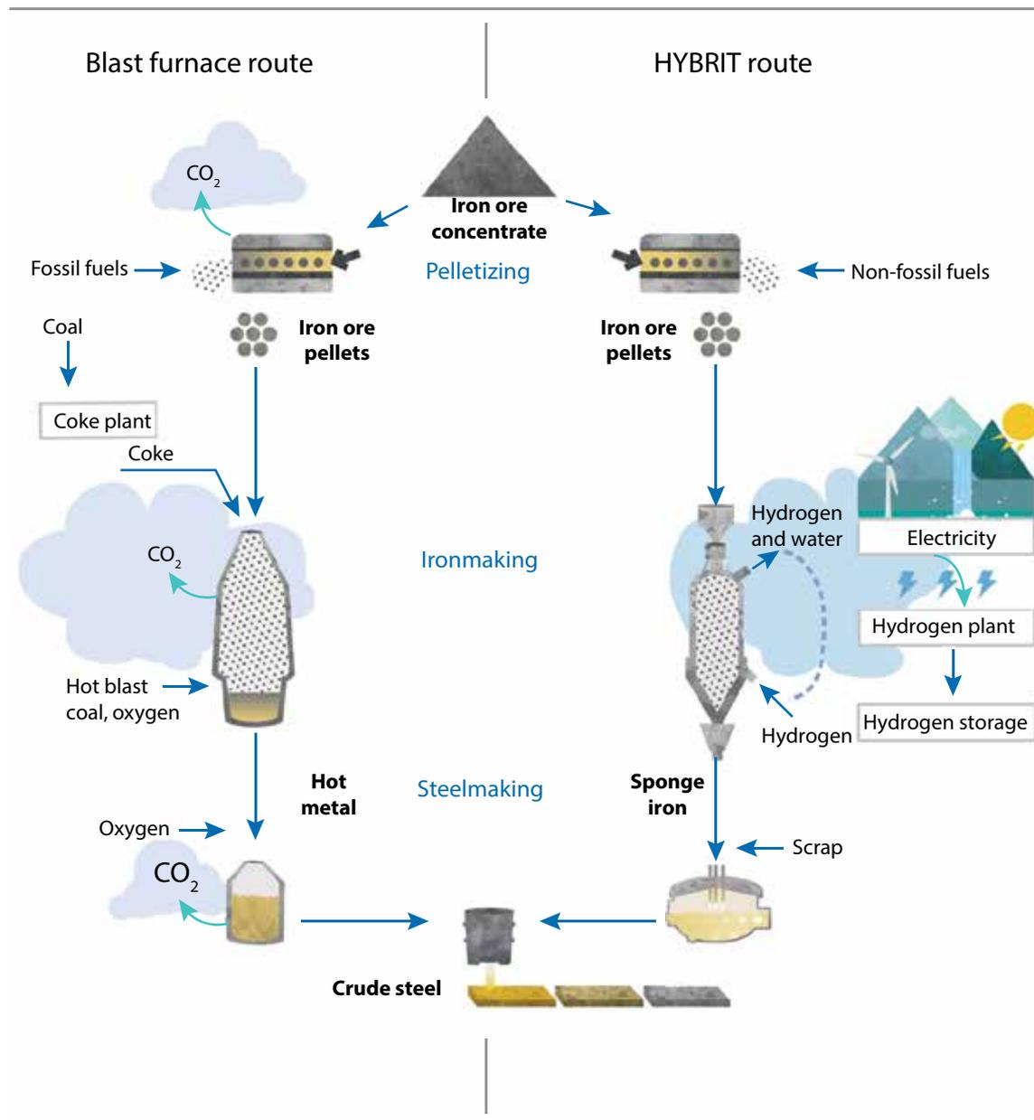
Comparison of blast furnace route and HYBRIT route
