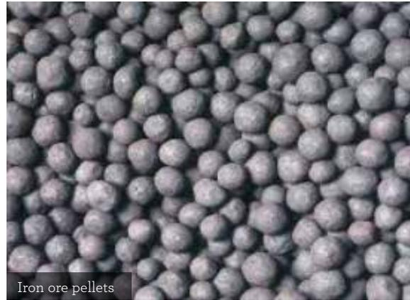
improved performance of the kiln. The use of iron ore pellets reduces loss on ignition. Two of the different iron ore pelletization processes are (i) straight travelling grate process and (ii) grate kiln process.
