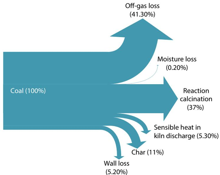
Typical energy balance of a coal-based rotary kiln
