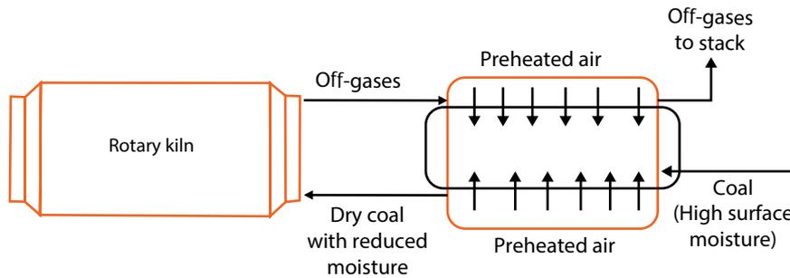
WHR-based rotary drum dryer for surface moisture removal for coal
