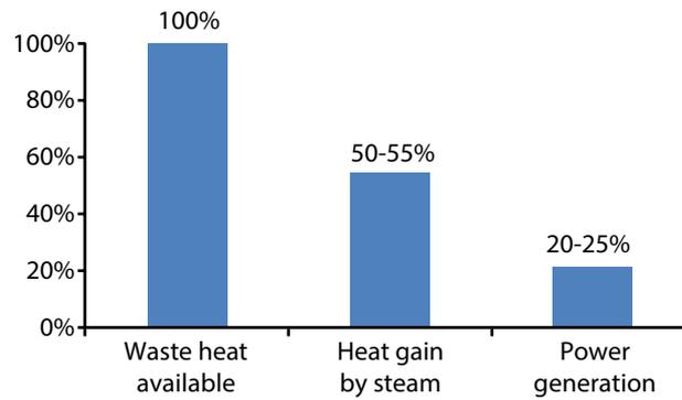
Waste utilization from rotary kiln
