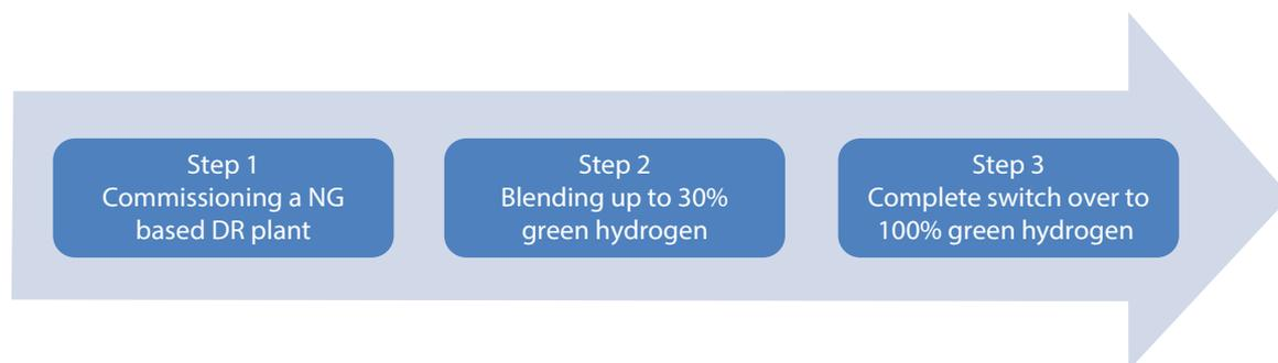
A stepwise approach to reduce CO<sub>2</sub> emissions via the direct reduction route.
