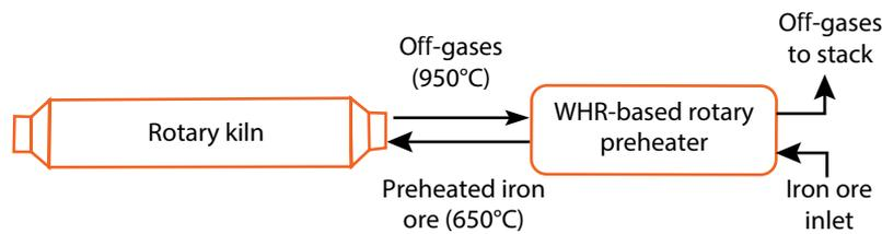
Preheating rotary kiln for iron ore using WHR system
