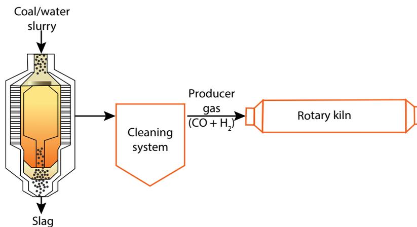
Coal gasification system for rotary kiln in sponge iron production
